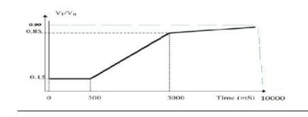
Provided that during the voltage dip, the supply of reactive power has first priority, while the supply of active power has second priority and the active power preferably be maintained during voltage drops, provided, a reduction in active power within the plant's design specifications is acceptable and active power be restored to at least 90% of the prefault level within 1 sec of restoration of voltage.
