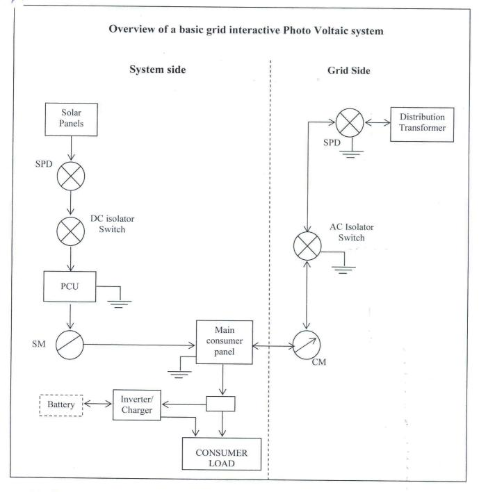
SPD- Surge Protective Device, PCU- Power Conditioning Unit, SM-Solar Generation Meter, CM- Consumer Meter (Net meter or Bi-directional meter)
