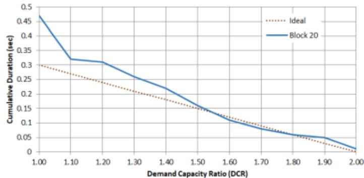
Figure 11 : Performance curve of point of changing slope in upstream face of Block 20 for time history analysis in DBE condition
