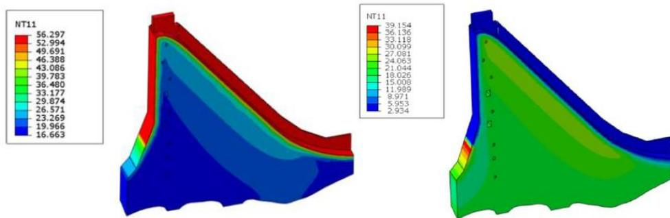
Figure 8: Temperature variation across Block 20 during extreme summer (on left) and extreme winter with lowest reservoir level.
