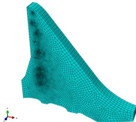
Figure 2: 3D Meshed Overflow section
