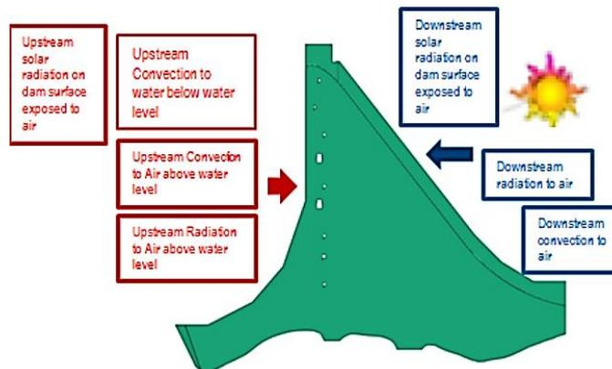
Figure 3: Physical processes of convection, conduction and radiation caused by thermal load (incident solar radiation) that are analyzed in the numerical model
