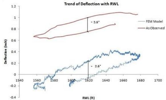
Figure 7: Trend of annual deflection due to RWL is seen to be a hysteresis with similar margin (~2.5inch) for both deflection series as observed in ground and from numerical model. This shows the numerical analysis is successful in capturing the effects of RWL.
