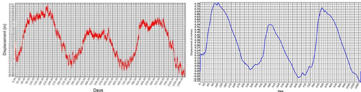
Figure 9: Deflection (inches) at plumb line point in Block 20 for load case in Scenario 1 - with (left) and without (right) thermal loads
