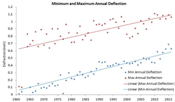
Figure 6: Plot of minimum and maximum annual deflections in observed at plumb line point of Block 20 from 1964. Over the years the values have slowly increased by about 4 inches
