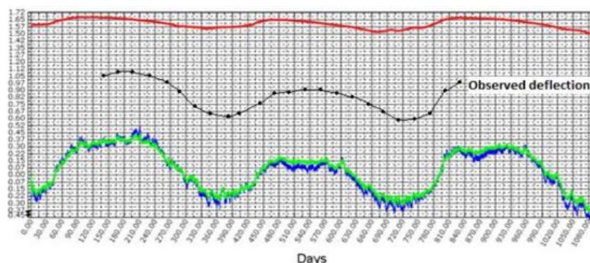
Figure 5: Comparison of deflections in Block 20 for simulation in Scenario 1. Deflection (inches) at the crest and plumb line measurement point of Block 20 are given in blue and green respectively. RWL in 1000ft (red) and observed deflection in inches (black line) are also indicated
