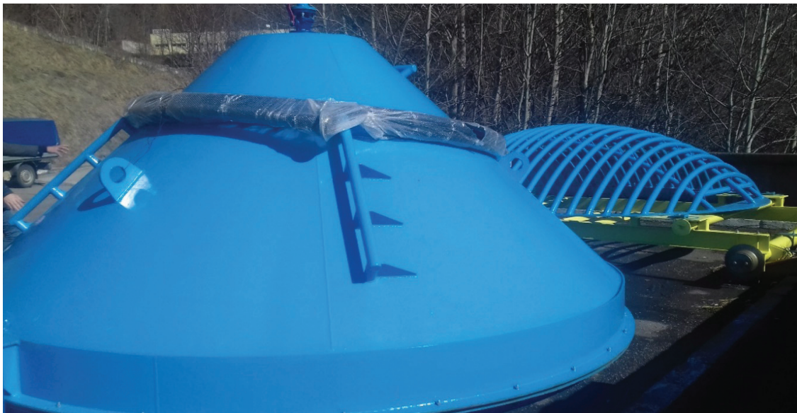
Figure 2 : The bell cofferdam and the new trash rack.
