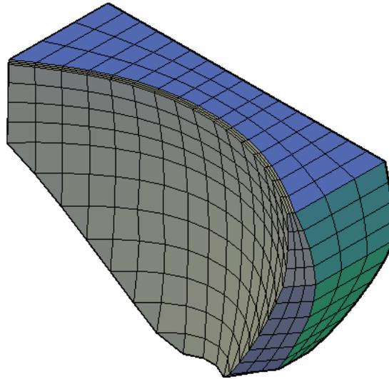
**Figure 1** : The finite element model of the Karun-3 dam
