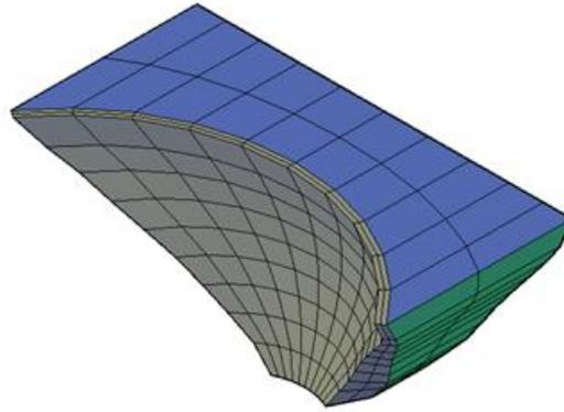
Figure 2 : The finite element model of the Karaj dam
