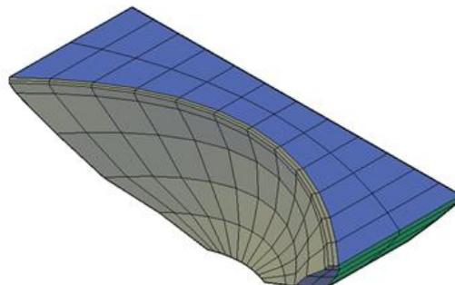
Fig. 3 : The finite element model of the Shahid Rajae dam
