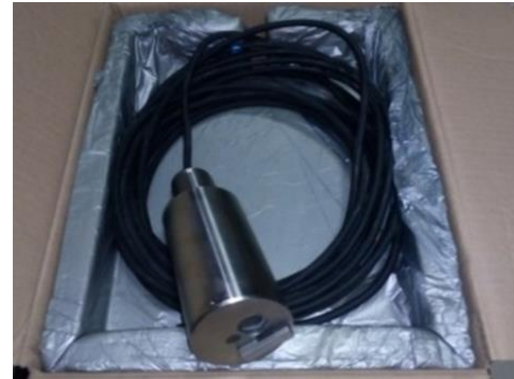
Portable Online Turbidity and suspended solids Sensor (Solitax)
