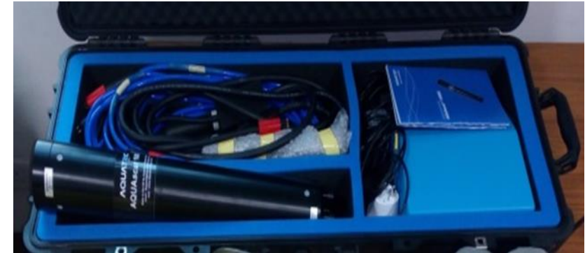
Online multi-frequency acoustic sensor (AquaScat)
