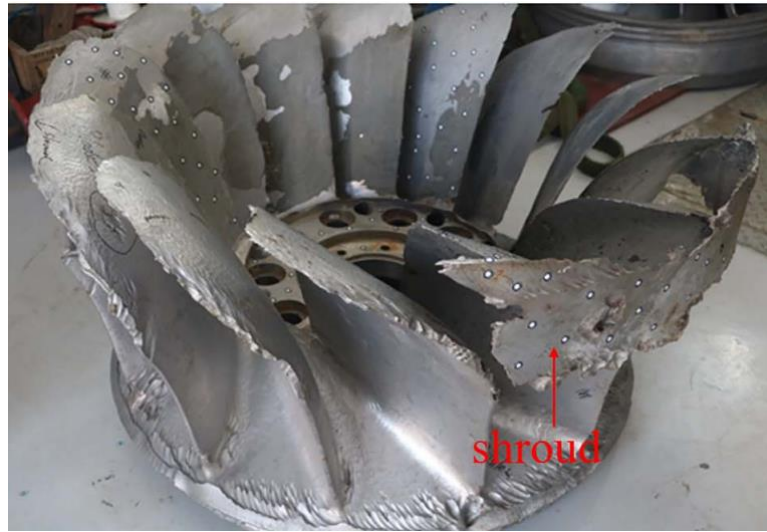
Eroded runner of Trishuli Francis turbine
