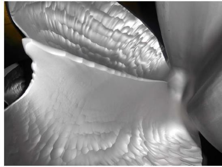
Eroded needle and bucket of Kashang Pelton turbine
