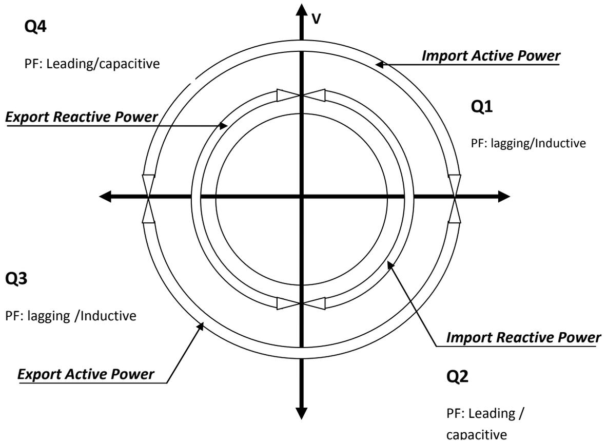
a. **Quadrant 1:** When current vector has an angle with voltage from 0 to 90 degree, power are to be referred in quadrant 1. Here, current vector is lagging from voltage vector with a certain angle. From start with zero angle, reactive component is zero. And at angle 90 degree angle, active component becomes zero. This quadrant represent that load is inductive.
