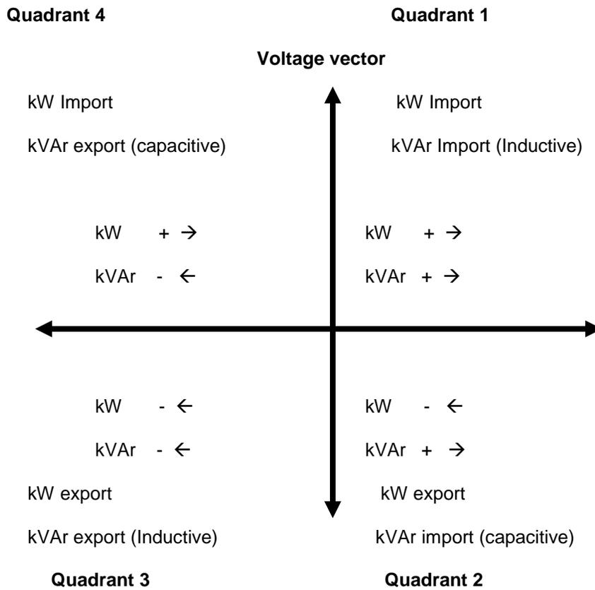
The power flow quadrant as per IEC 62053-23 is shown below.
