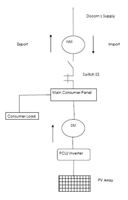
Normally, Solar Generation shall be connected with Grid. When grid fails, Inverter controlled Switch S3 Opens and on restoration of grid S3 Closes.
