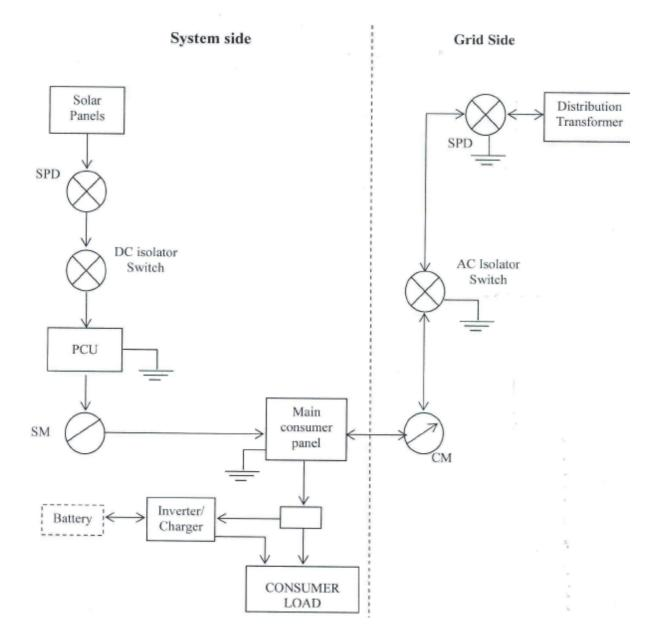
SPD- Surge Protective Device, PCU- Power Conditioning Unit, SM-Solar Generation Meter, CM-Consumer Meter (Net meter or Bi-directional meter)
