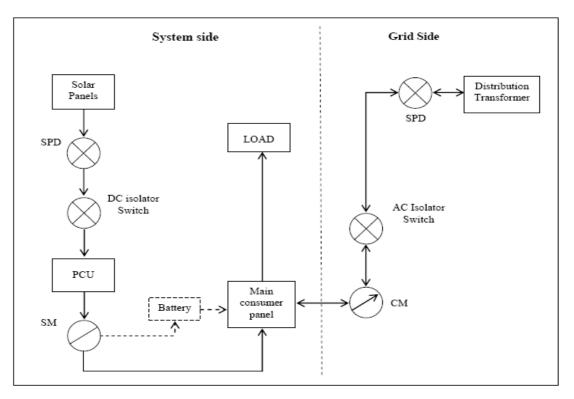
SPD- Surge Protective Device, PCU- Power Conditioning Unit, SM-Solar Generation Meter, CM- Consumer Meter (Net meter or Bi-directional meter)
