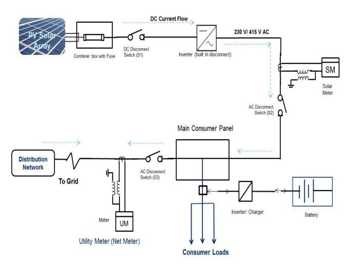
The utility meter (Net-meter) has to be bi-directional meter to register both import grid electricity amount as well as export solar electricity amount
